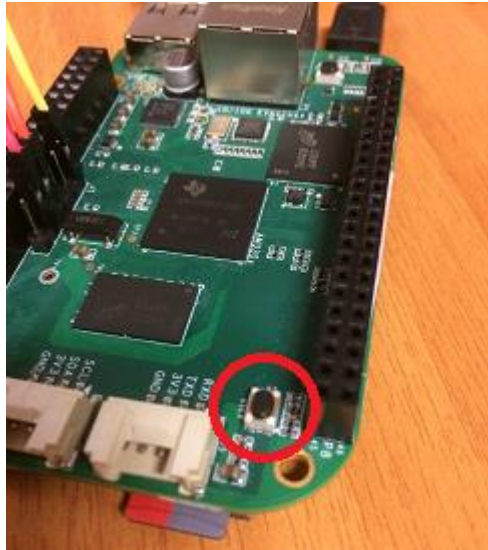
Figure 16: Button to press during power-up in order to switch the boot source to the uSD card.
